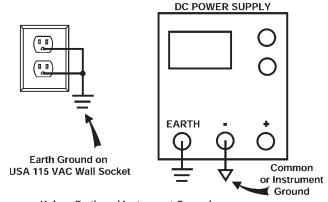
Unless Earth and Instrument Ground are connected via the power supply, Instrument Ground is floating with respect to Earth Ground.
