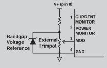
(1) An external trimpot or potentiometer can be attached to pin 3 to remotely control the laser diode current.
